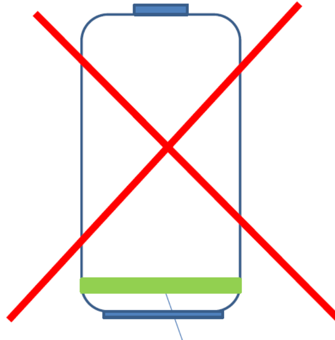
Discharging cell until empty damages cells and reduces life time
